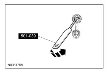
4. Using the Power Point Socket Remover, pull the power point socket out of the retainer.
