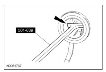
3. Position the Power Point Socket Remover so that it engages in the adjacent slot.
